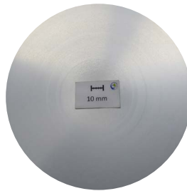
Macrosection, d178 mm: Segregation zone 2,7 mm
