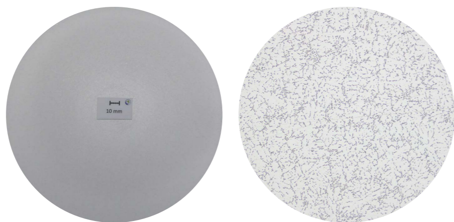
Macrosection, d252 mm: Segregation 3,1 mm Microsection, d252 mm (25 times magnification)
